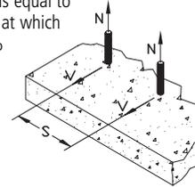
Notes: For anchors loaded in tension, the critical edge distance ( $c_{cr}$ ) is equal to 12 anchor diameters ( $12d$ ) at which the anchor achieves 100% of load.
