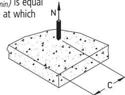
Notes: For anchors loaded in shear, the critical edge distance ( $c_{cr}$ ) is equal to 12 anchor diameters ( $12d$ ) at which the anchor achieves 100% of load. Minimum edge distance ( $c_{min}$ ) is equal to 5 anchor diameters ( $5d$ ) at which the anchor achieves 50% of load.
